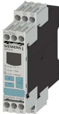
Digital monitoring relay for residual current monitoring (with current transformer 3UL23) Setting range 0.03...40 A separate for warning threshold and switch-off value supply voltage 24 ... 240 V AC/DC, 50 .. 60Hz ON delay and tripping delay 0.1 to 20 s Shutdown hysteresis up to 50% Warning hysteresis 5% fixed Width 22.5 mm, 2 change-over contacts with or without fault buffer screw terminal
