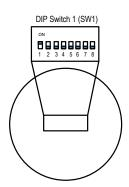
**Input channel select**–Use switch positions 1 through 6 on SW1, to select the channel that would be used to operate the audible module. Switch positions 7 and 8 are not used.
